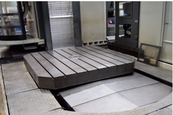
Mesa Roto-Translante / Roto-traversing table: BOST mod. ZA/B-2000 2500 x 2500 mm (2008)
